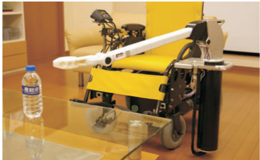
RAPUDA attached to an electric wheelchair
